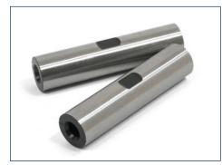
Rifle drilled 8620 Kin pins are hardened and ground for wear resistance and feature a set screw flat for positive locking.
