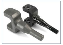
The Heat Treated Chromoly Spindle starts life with and American produced forging. Each Spindle is individually hardness tested and 100% Magnaflux inspected.
